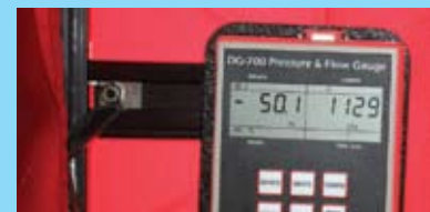
The blower door reading after Spray Insulation had completed its work showed an air exchange of 1,130 CFM, a reduction of more than 20 percent in air infiltration.
